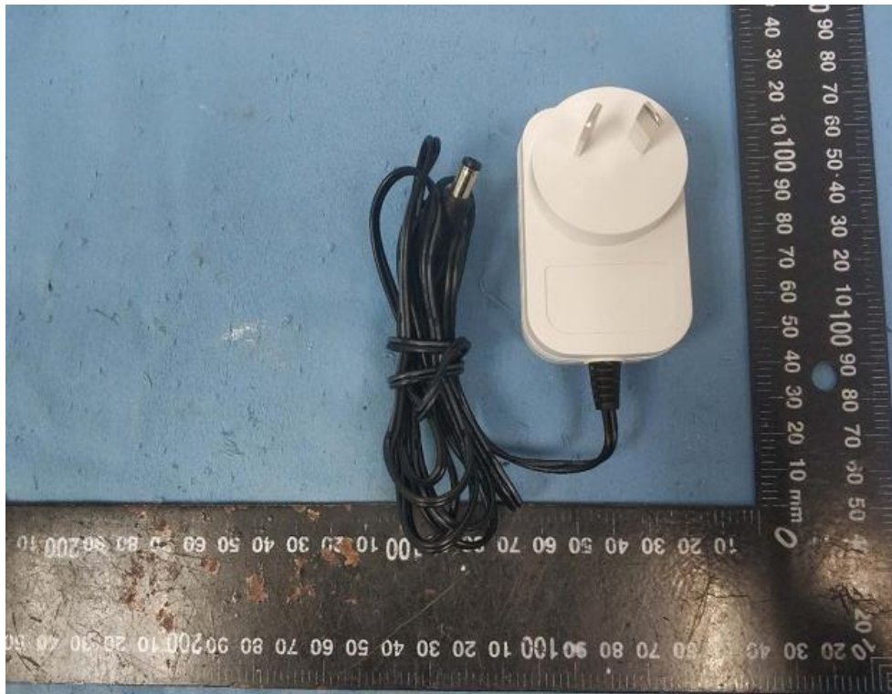
External view of the appliance for models 18W series with SAA plug and output cord output
