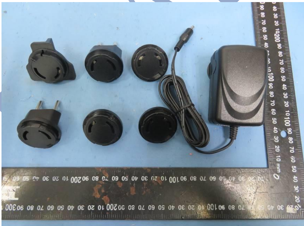
External view of the appliance for models 36W series with Detachable plug
