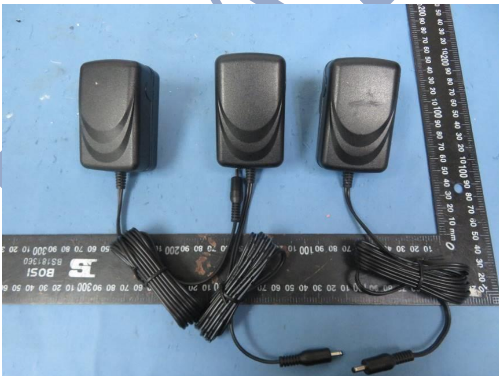
External view of the appliance for 36W series models with output cord
