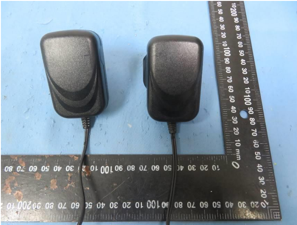
External view of the appliance for models 18W series with fixed plug and output cord output
