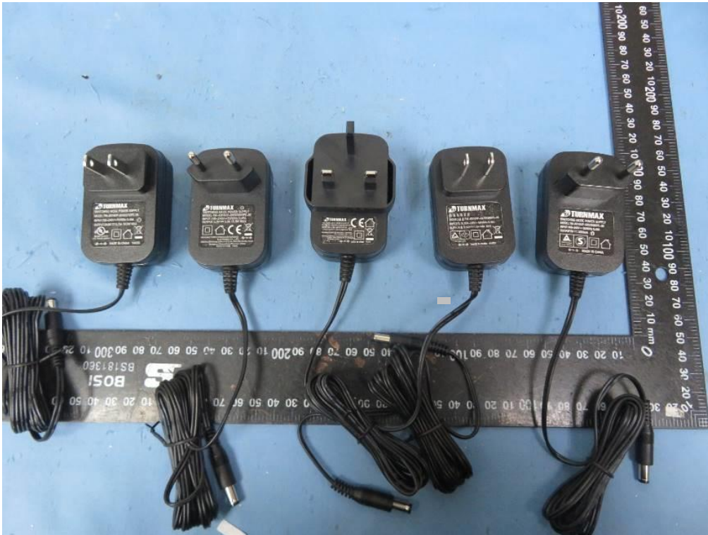
External view of the appliance for models 18W series with fixed plug and output cord output
