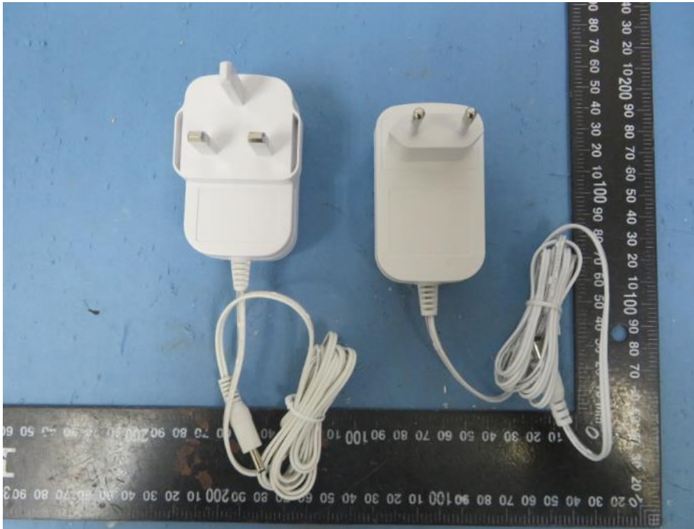
External view of the appliance for 24W series models with output cord
