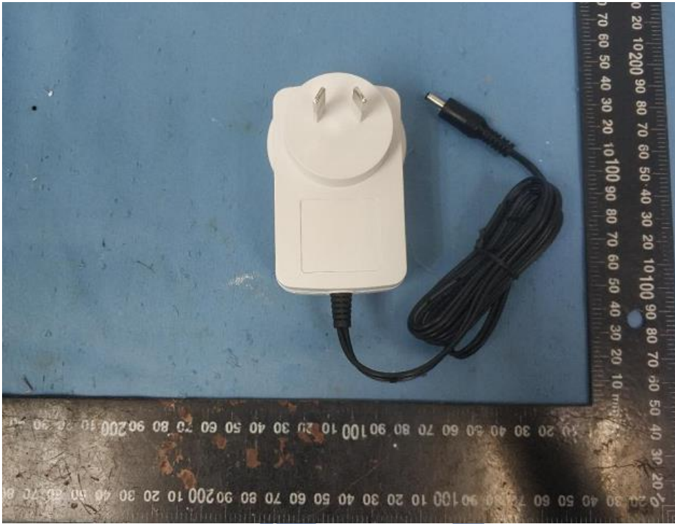
External view of the appliance for 36W series models with output cord
