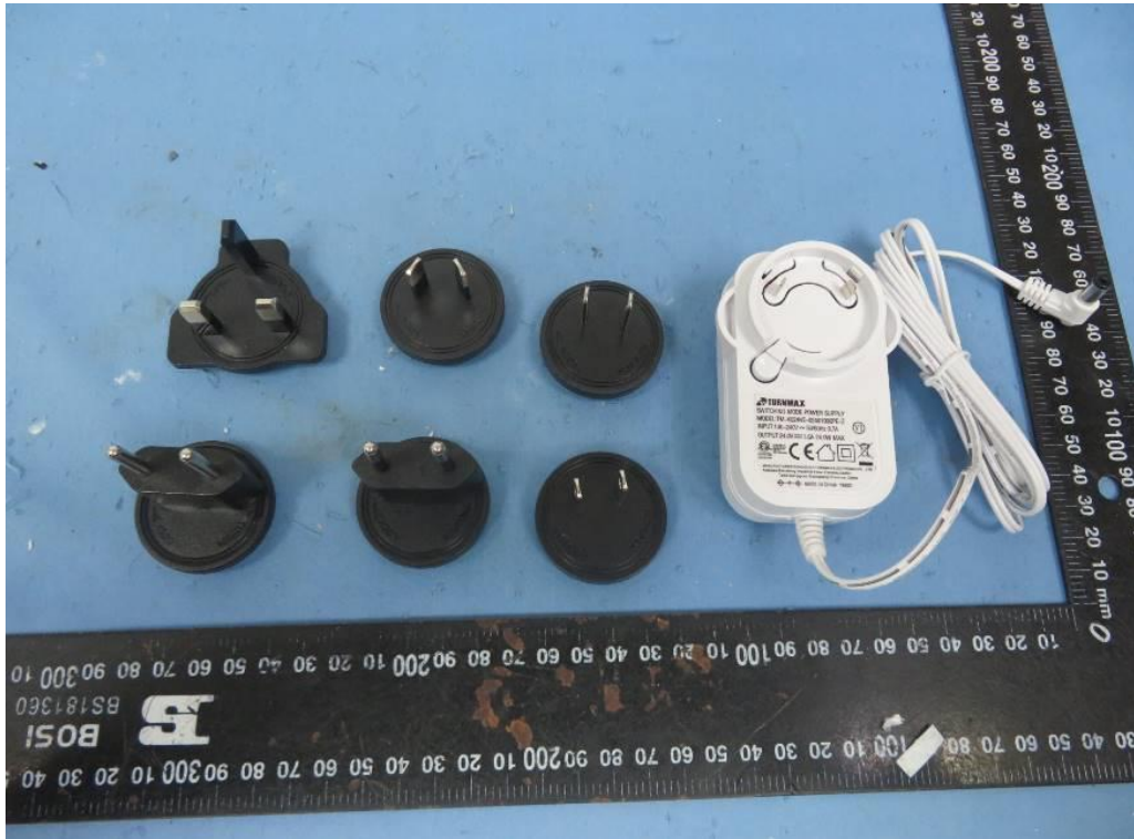
External view of the appliance for models 24W series with Detachable plug
