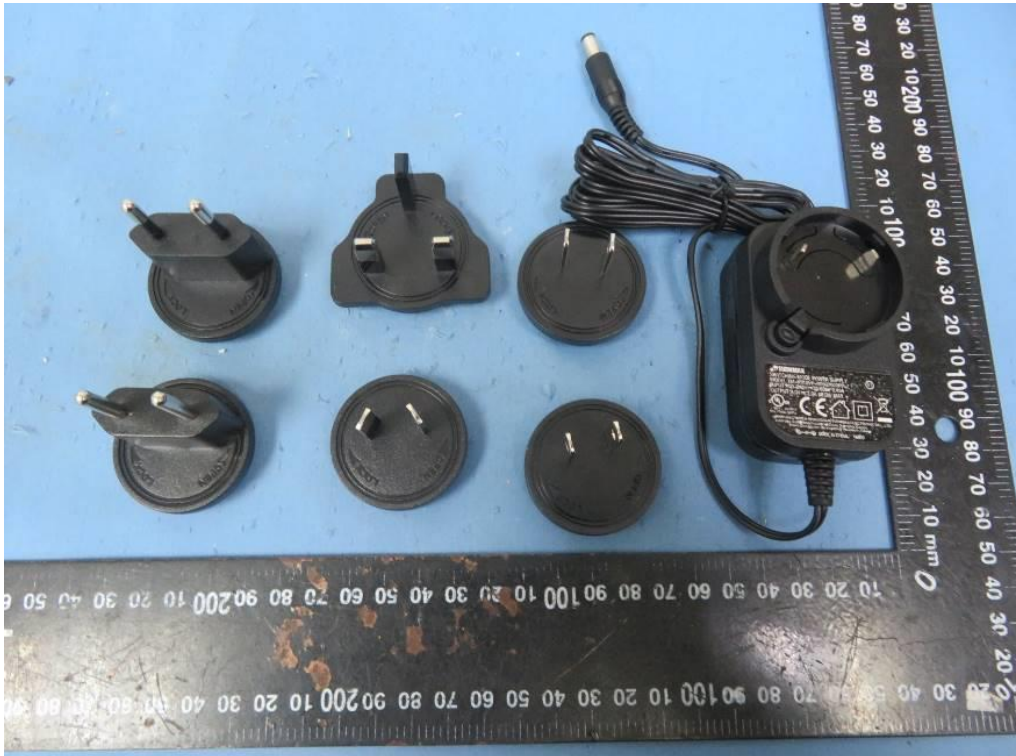
External view of the appliance for models 18W series with Detachable plug
